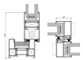
The XS-60 system has been designed to provide a minimalist and functional solution for building projects. Its central node of only 35 mm and its 60 mm section make it an optimal solution both for new construction and for the refurbishment of old buildings.
