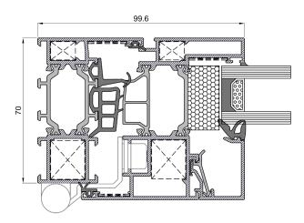
The XP-70+ system, 70 mm of section, standard 16 groove hardware and 34 mm thermal breack, provides excellent thermal and acoustic performance. It is designed for modern architecture allowing large windows without compromising on performance.
